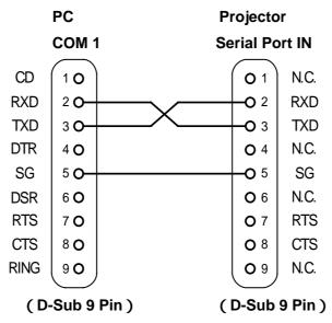
Connect COM port of a computer to SERIAL PORT IN of a projector.
