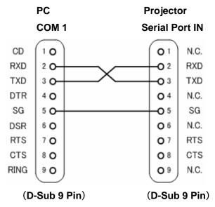
Connect COM port of the computer to SERIAL PORT IN of the projector.
