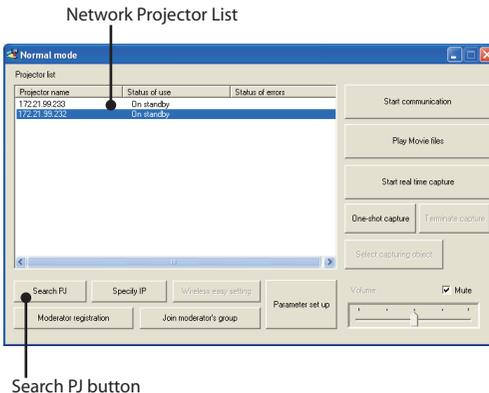
When set up the projector in the location separated by the router and the segment is different; Projector will not be found nor displayed. In that case, the projector needs to be searched directly by the IP address.
