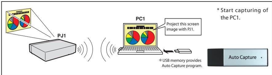
The real time capture function can run automatically on the computer without the Network Viewer & Capture 5 software installed by executing the Auto Capture program in the USB thumb drive connected to the computer. The USB thumb drive for Auto Capture is supplied with this projector.
