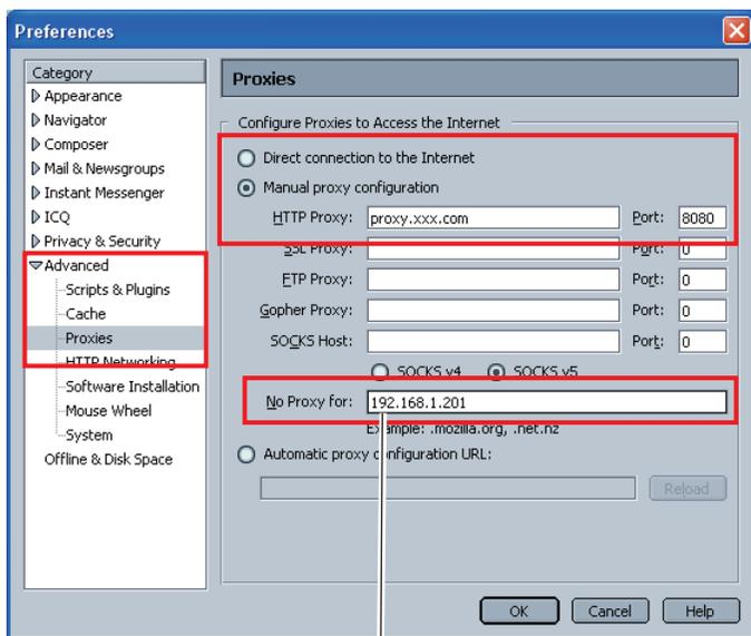
To designate proxy settings that will not use the proxy server when accessing the projector installed in the local area network, enter the IP address or domain name here.
