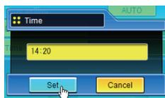
This projector does not provide the built-in battery. The date and time information are lost when the projector turns off ( when "Eco" is set for the stand-by mode (Refer to p.74)), or the network configuration is reset. The timer function is disable until time is set up correctly. When using the NTP address for time setting, the current time is acquired at the projector starting up and the timer function is activated after finishing the time setting correctly.
