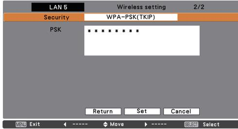
2. Use the Point ▲▼ buttons to select the key field and press **SELECT** button. The PSK key entry screen appears. Enter the PSK key by using the Point buttons. If the input PSK key has an error, the PSK key is indicated in red.
