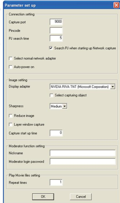
☞ To check the Capture Port number, see item "Control by the web browser" (☞ p.93). To check the PIN code, see item "Network PIN code setting" (☞ p.32, p.42).
