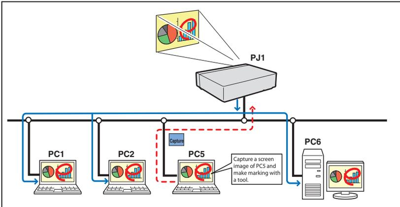
\*The Main PC is a computer which started using communication function, and serves own computer screen captured image to the Sub PC. The Main PC has an authority to quit using whole communication. To become the Main PC, execute the command "Start Communication" or "Capture transfer". For further information, see item "How to use the Network Communication". (p.100)
