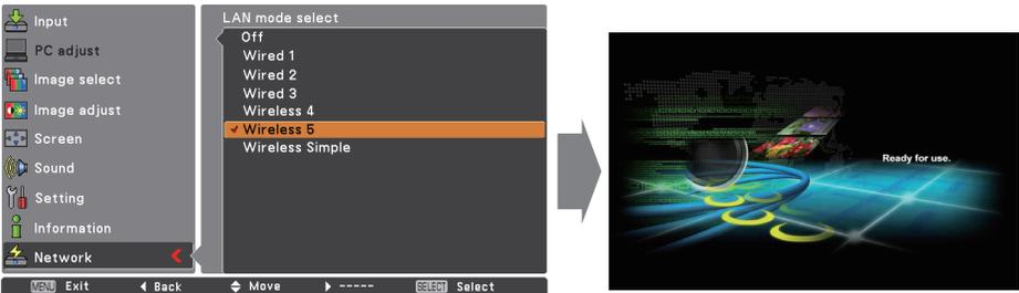
4. Select "Network setting" in the Network menu and press **SELECT** button, and then the LAN setting screen will appear and the selected LAN settings will be displayed. Adjust each item to the setting environment. Consult your system administrator for the detailed settings.
