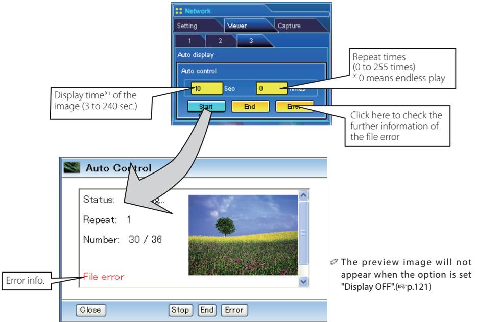
1. Click **Start** button to start the auto-display. The image in the selected folder or program is displayed on the projector's screen. The web browser opens another window and displays the preview images on the Auto Control window sequentially.
