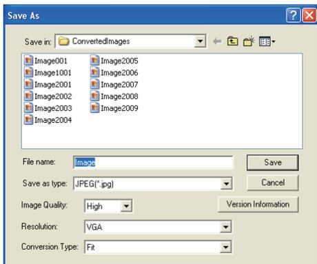
☞ The file name is named with "Image001" as default. If the converted image has 2 or more pages, the file names are numbered from "001" to "999" in serial order.
