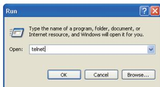
2. The telnet application will start and the following window will be displayed. Type as below to connect the projector.
