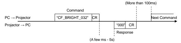
When a computer sends next command before receiving a response, the projector may not operate properly, except when there is no response for more than 5 seconds.
