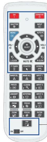
Only these buttons are active when the simple mode is set to **On**. [ON, STAND-BY, SHUTTER, INPUT, MENU, AUTO PC, SCREEN, ▲, ▼ (MUTE), ◀ (VOLUME-), ▶ (VOLUME+), SELECT (Mouse Pointer included), L-CLICK, R-CLICK, P-TIMER, POINTER, PIP, ON-OFF switch] Number buttons (p.14) also become active only when setting the remote control codes numbers or entering the PIN code numbers (pp. 54, 62).
