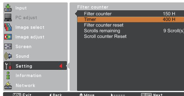
Press the SELECT button to select **Timer** and then use the Point ▲▼ buttons to set the timer. Select from (**Off/400H/700H/1000H**) depending on the use environment.
