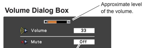
Press the Point ▼ button to set the Mute function **On** or **Off**. The dialog box disappears after 4 seconds.
