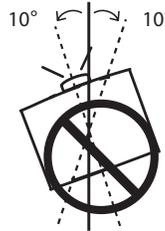
In upward projection, do not tilt the projector over 10 degrees right and left.
