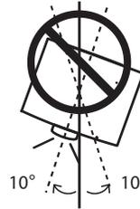
In downward projection, do not tilt the projector over 10 degrees right and left.
