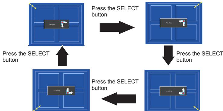
Reduce the bottom left corner part with the Point ▶▲ buttons.
