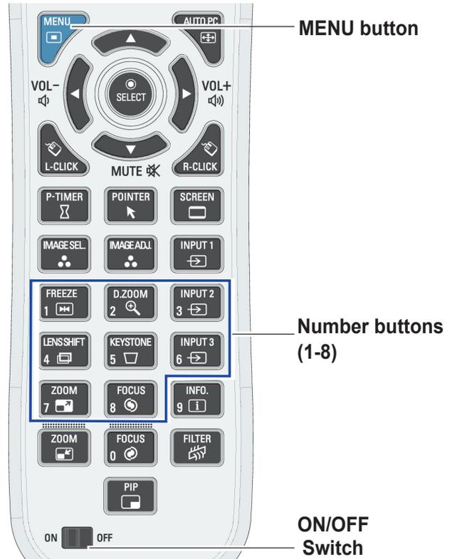
Press and hold the MENU and a number button (1-8) that corresponds to the remote control code for more than five seconds to switch between the codes.
