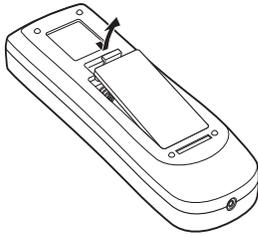
**2** Install new batteries into the compartment.
