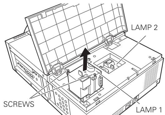
Make sure which number of lamp needs to be replaced on Lamp Status Display. Figure shows case of replacing LAMP 1.
