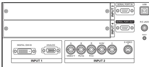
DVI / D-sub 15 Terminal    5-BNC / VideoTerminal
