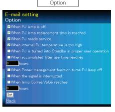
"When PJ lamp is off" signifies the lamp goes out without user operation. "When PJ is turned into Standby in proper user operation" signifies that the projector is turned on by using the web browser and then it is turned into standby with ON/STANDBY button on the top control or the remote control.
