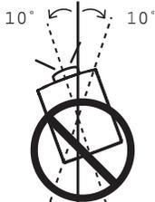
In upward projection, do not tilt the projector over 10 degrees right and left.
