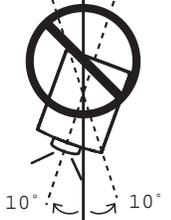
In downward projection, do not tilt the projector over 10 degrees right and left.
