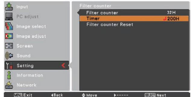
Press the SELECT button to select **Timer**, and then use the Point ▲▼ buttons to set the timer. Select from (**Off/ 100H/ 200H/ 300H**) depending on the use environment.
