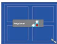
Reduce the bottom left corner part with the Point  $\blacktriangleright$   $\blacktriangle$  buttons.
