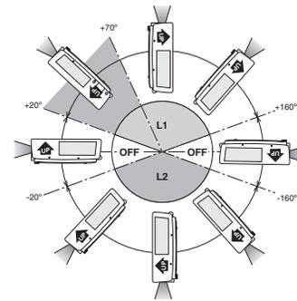
\* When installing the projector in upwardly inclined position, install the projector bottom side up.
