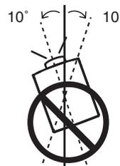
In upward projection, do not tilt the projector over 10 degrees right and left.
