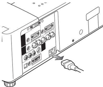
2 Remove the connector cover and screw covers (2 pieces) from the projector and insert plug on this product to the option connector.
