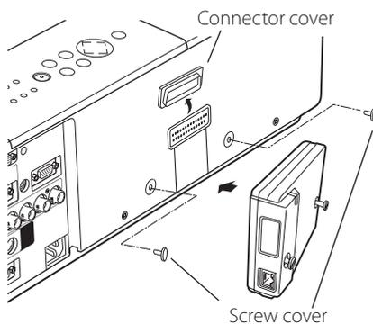
3 Tighten two screws by using a coin etc.
