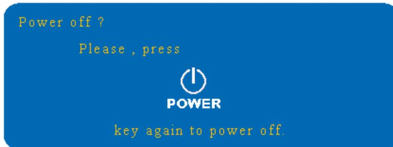
2. Press the power button again and the projector will enter cool-down mode. The lamp shuts off, the lamp indicator flashes red, and the fans continue to run for approximately two minutes. During the cool down sequence the projector will not respond to any control panel or remote control buttons.
