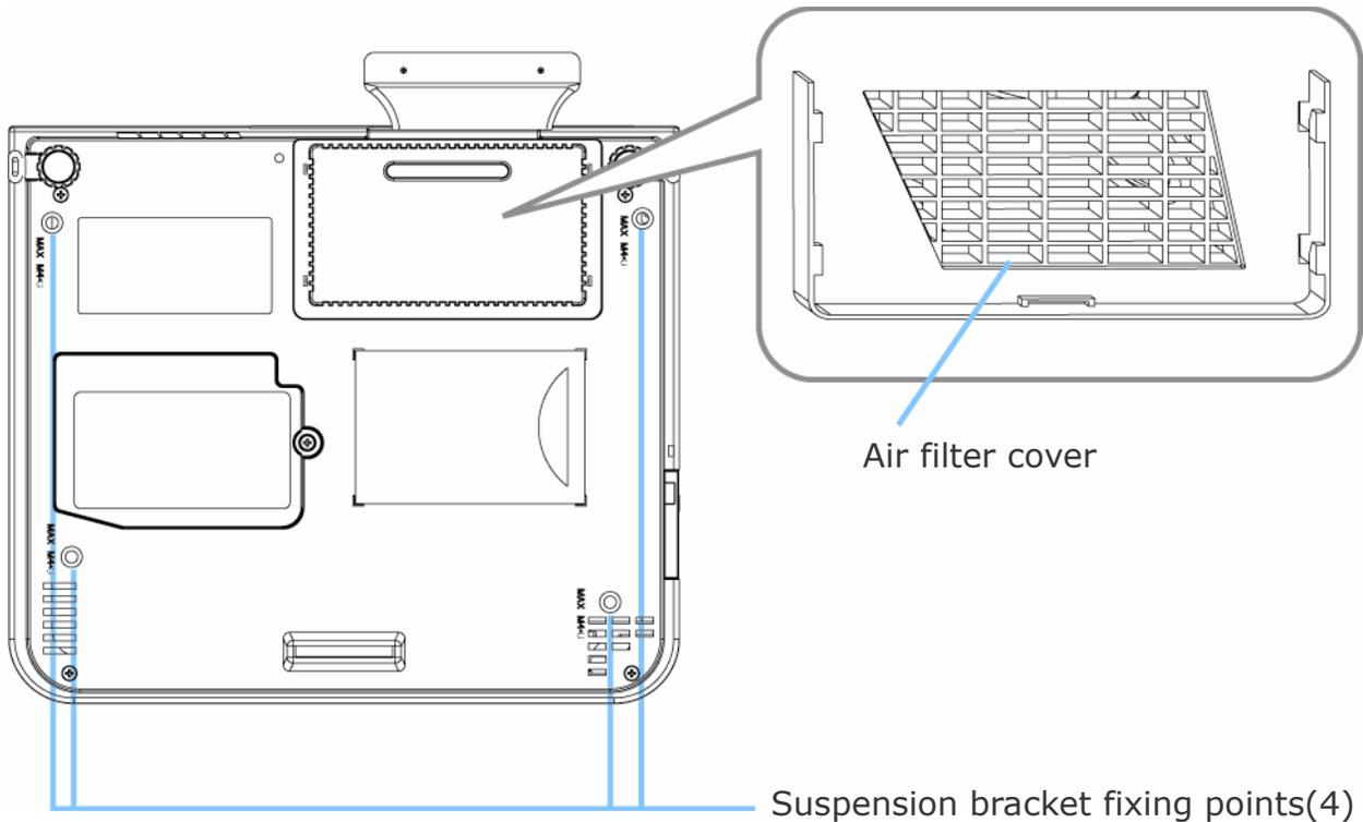
**1. Suspension bracket fixing points (4 points)**
