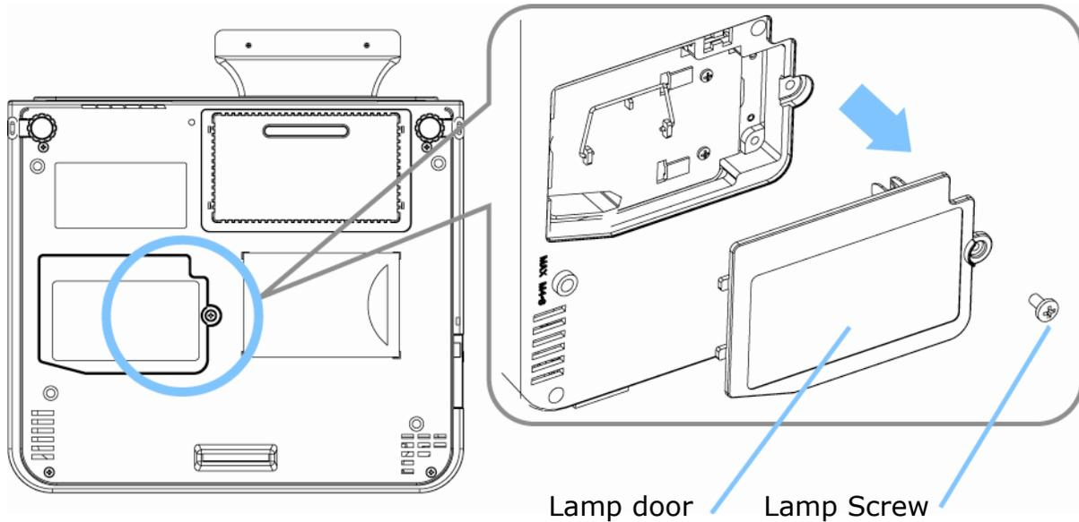
1. Remove the lamp screw from the lamp door.
