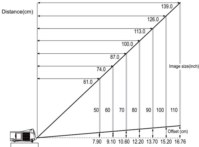
When installed against a wall, leave about 20cm (7.9in.) between the projector and the wall. Please see the detail of the minimum required space on page 6.
