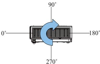
The projector can be installed pitched by any angle (360 degree) without any setting in fan mode. As for rolling it must be within 10 degree.
