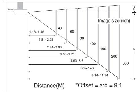
When in against at wall, leave about 20cm (7.9in.) between the projector and the wall.
