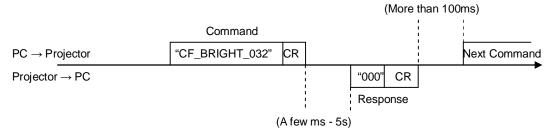
When a computer sends next command before receiving a response, the projector may not operate properly, except when there is no response for more than 5 seconds.
