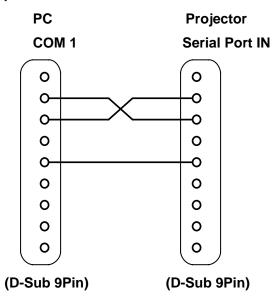
Connect COM port of the computer to SERIAL PORT IN of the projector.
