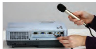
Mic input for P/A or Voice-over.
