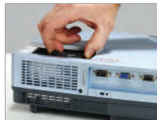
Top-accessed lamp compartment.
