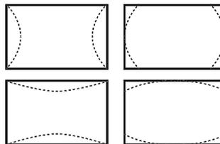
Geometric correction adapts the image for projection on a spherical, cylindrical and other specially shaped screens.
